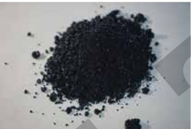
搪玻璃底釉釉块 The frits for ground coat enamel
